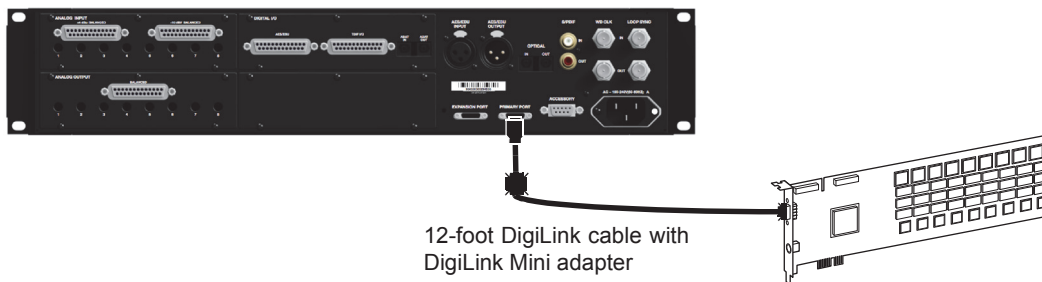
Figure 5. HD I/O connected to the DigiLink Port on a Pro Tools|HD Accel Core card (16-channel I/O system)
