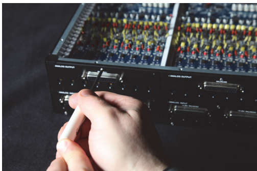
Removing the screws securing an I/O card
