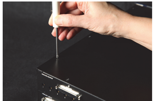
Removing the top cover screws
