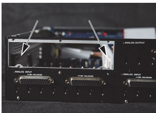
Guide rails along sides of empty bay
