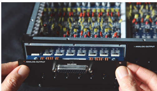
Removing an I/O card from the HD I/O chassis
